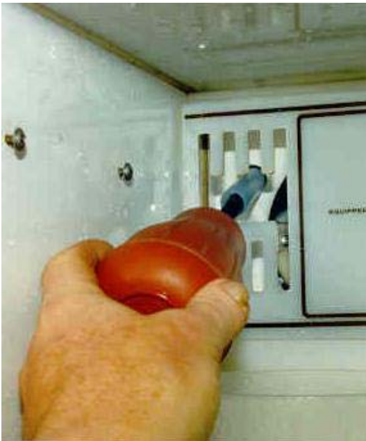
Fig. 09-06 Thawing a Frozen Spout
