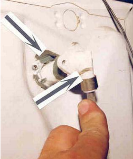
Fig. 09-04 A Cracked Icemaker Spout Being Replaced
